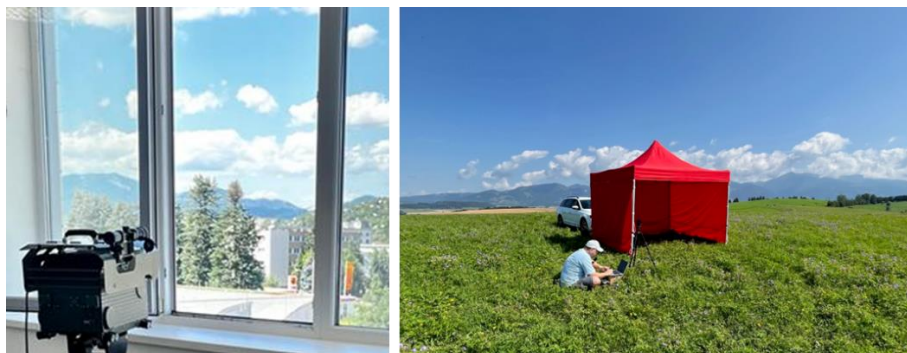
Figure 2.6: Falcon 4G (left) pointed on a tent installed on hill side for open air releases (right).
