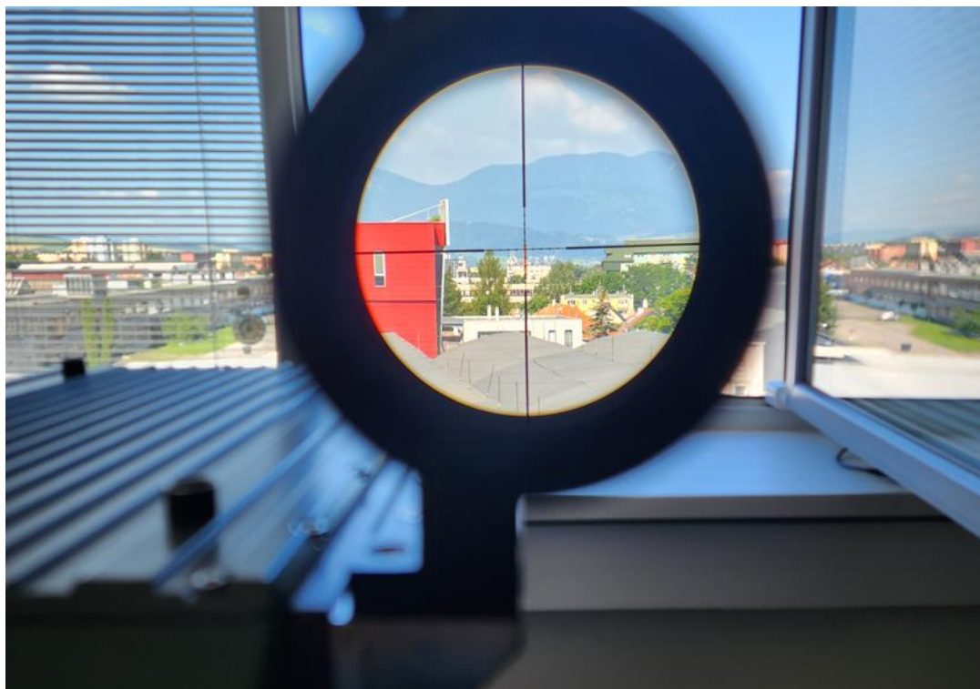
Figure 2.4: A scope was used to aim the detector to a reflecting background, in this case a chimney at 1750 meters.
