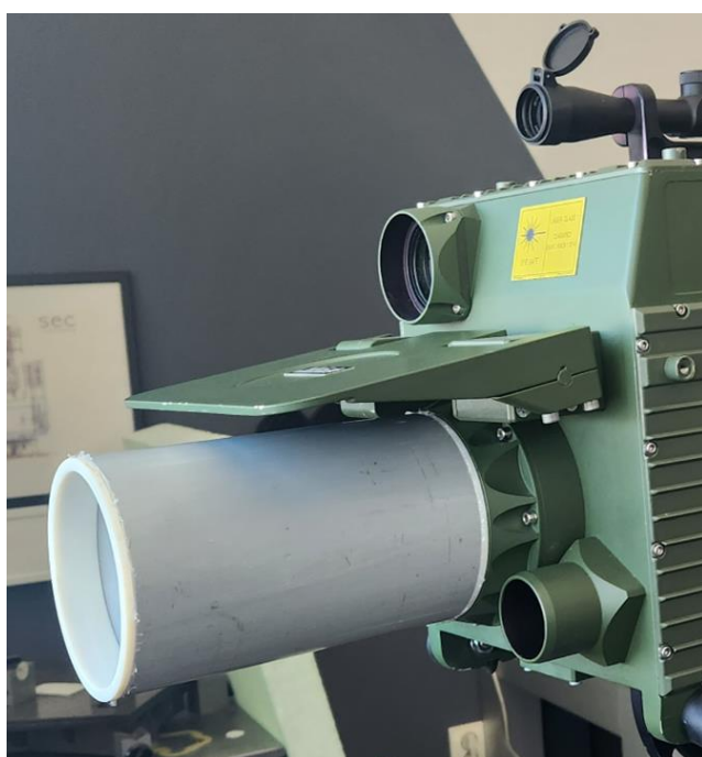
Figure 2.5: Gas Cell (PVC tube) installed in front of the Falcon 4G ‘detector’ optical receiver.
