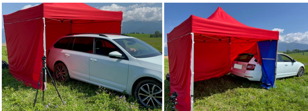
Figure 2.7: Creating a diesel exhaust background in the tent.
